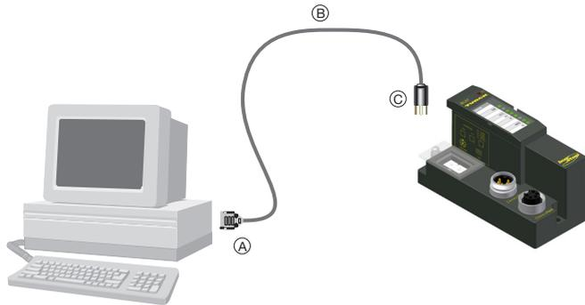
Fig. 9: BL67-gateway connected to PC via special cable
