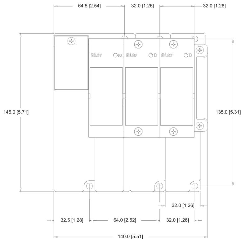
Fig. 4: Dimensions/drilling plan
