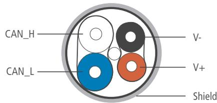
Fig. 39: DeviceNet cable schematic
