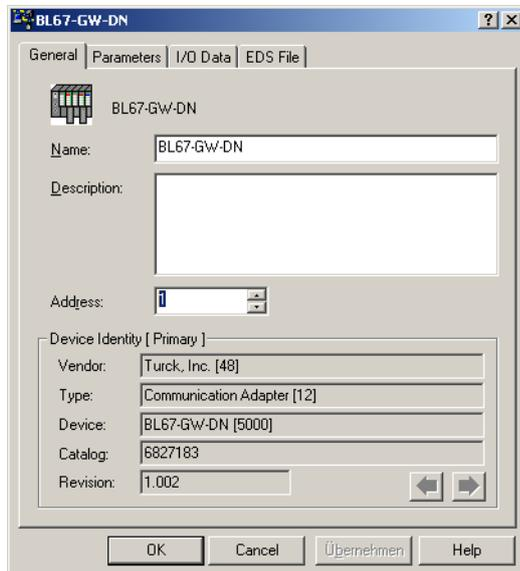
Fig. 26: Setting the node address of the BL67 gateway
