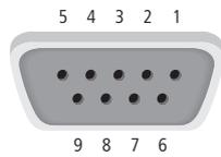
Fig. 11: 9-pole SUB-D female connector on the cable for connecting to PC (top view)
