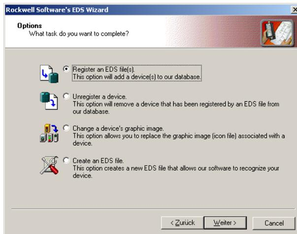
Fig. 23: Registering the EDS File
