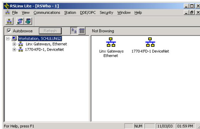
Fig. 21: Depicting the DeviceNet network in RSLinx
