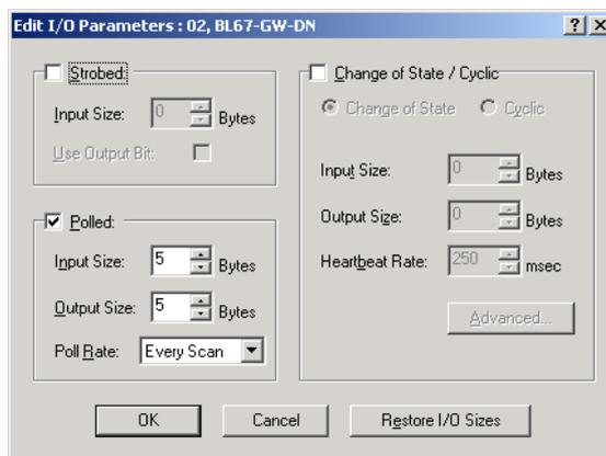
Fig. 31: Setting the type of data transmission
