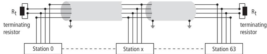
Fig. 38: Representation of a bus cable
