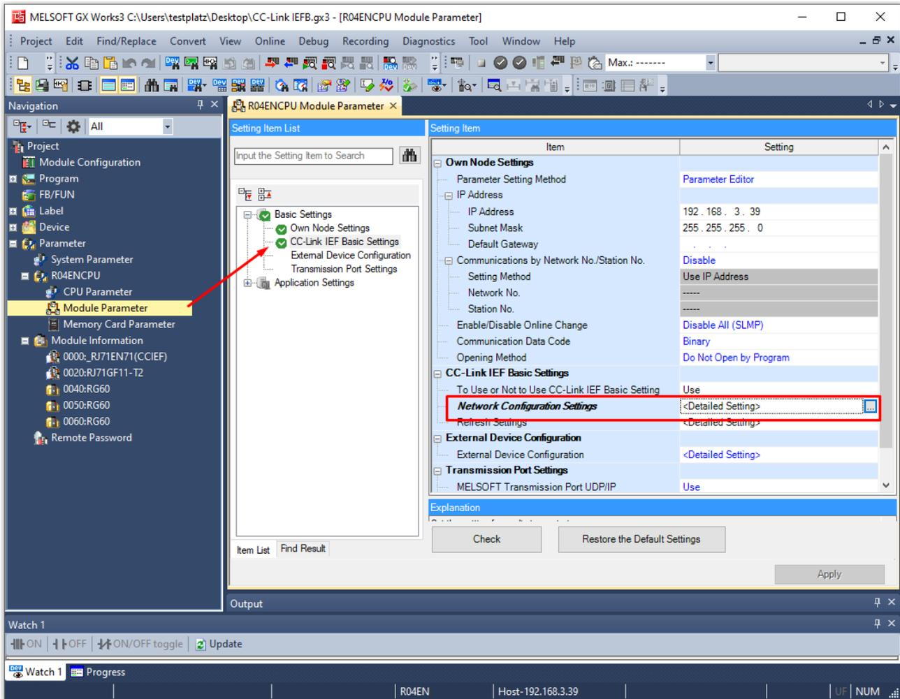
Abb. 74: GX Works3: Network Configuration Settings
