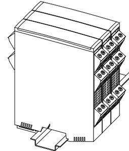
IMX12-TI ...-...-0/... mount directly on the DIN rail.
