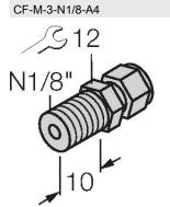
9910406 Compression fitting for direct mounting of temperature sensors; sensor diameter 6 mm; process connection 1/8" NPT male thread
