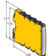
Isolating switching amplifier, 2-channel; SIL2 acc. to IEC 61508; Ex-proof version; 2 transistor outputs; input Namur signal; ON/OFF switchable monitoring of wire-break and short-circuit; toggle between NO/NC mode; signal doubling; removable screw terminals; 12.5 mm wide; 24 VDC power supply
