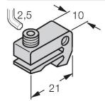
Mounting bracket for mounting magnetic field sensors on profile cylinders (IMI Norgren); cylinder diameter: 32...100 mm; material: Anodized aluminum
