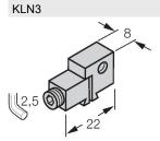
Mounting bracket for mounting magnetic field sensors on dovetail groove cylinders or T-groove cylinders; clamping width: 5.2... 13.5 mm; material: Anodized aluminum
